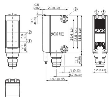
Figure 36: Dimensional drawing - FlexChain GL6-C
