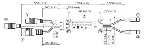
Figure 2: Sample view of FlexChain Host CANopen variant
