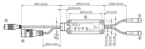
Figure 34: Dimensional drawing – FlexChain Host Standard
