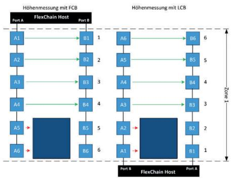
Figure 19: Height measurement FCB/LCB
