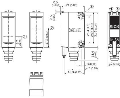
Figure 37: Dimensional drawing - FlexChain GSE6-C
