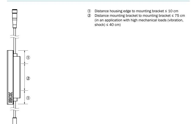
Figure 32: Mounting bracket and mounting distance
