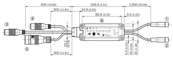
Figure 35: Dimensional drawing - FlexChain Host CANopen
