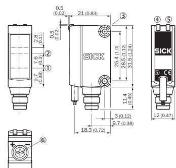
Figure 38: Dimensional drawing - FlexChain GSE6-C
