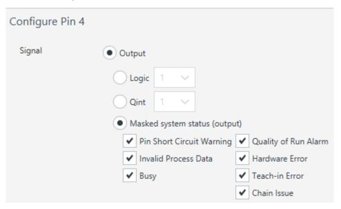
Figure 31: Configuration of PIN 4 / Masked System Status
