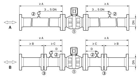
Installation of the FLOWSIC600-XT in the pipeline for bidirectional use (minimum requirements)
