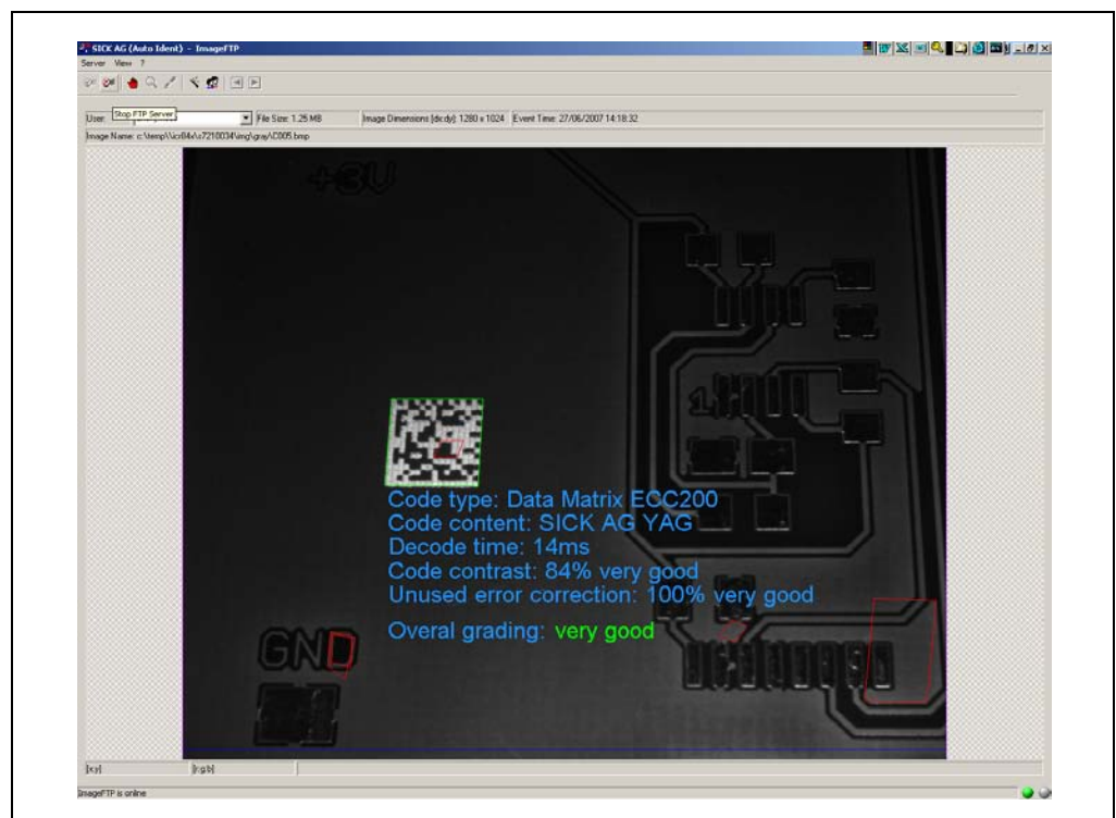
Fig. 6-13: ImageFTP: Image presentation mode, here with reading diagnosis data for the code
