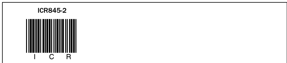
Fig. 6-19: Bar code sample (code 39; module width 0.35 mm (13.8 mil); print ratio 2:1)
