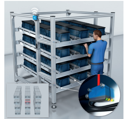
Automated material reordering at e-Kanban racks
