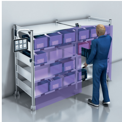
2D-LiDAR-based shelf monitoring at the smart shelf
