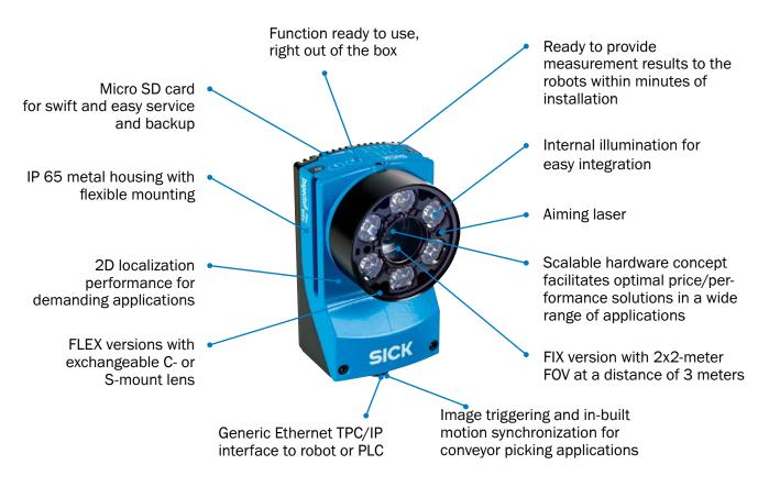
The PLOC2D is a vision sensor system for the localization of parts in 2D. The system is equipped with a high-quality imager combined with a high-performance localization algorithm for reliable and fast part localization. The sensor system is
