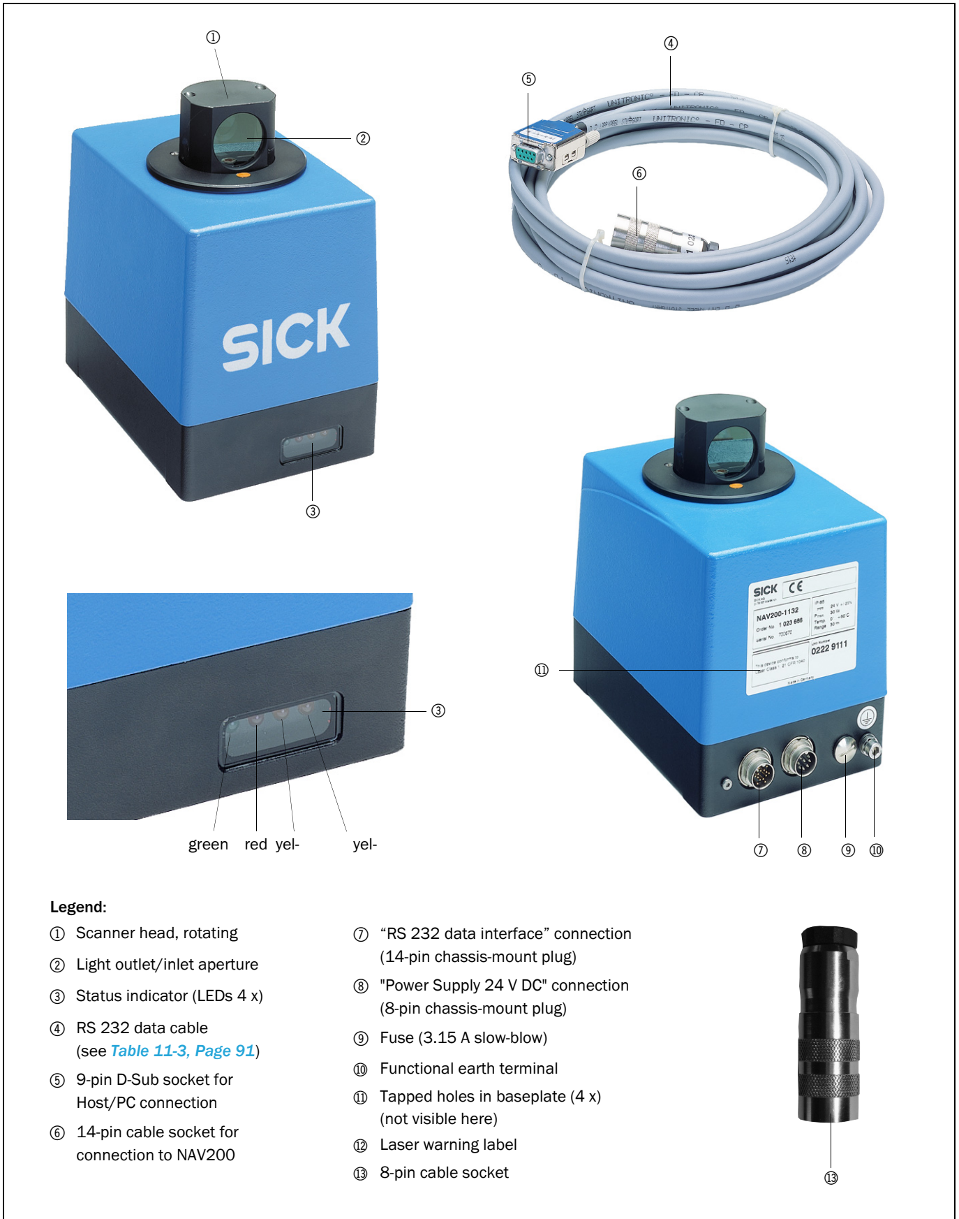
Fig. 3-2: Arrangement of the NAV200
