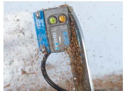
BluePilot: The shorter the distance of the blue LEDs from each other, the higher the degree of contamination is (e.g., RAY10)
