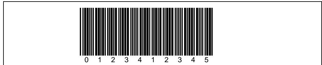
Fig. 6-1: Bar code sample (code 39; module width 0.35 mm; print ratio 2:1)
