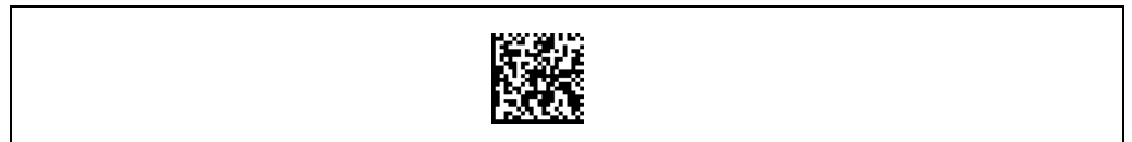
Fig. 6-1: 2-D code sample (DataMatrix ECC200; cell size 0.3 mm (11.8 mil))
