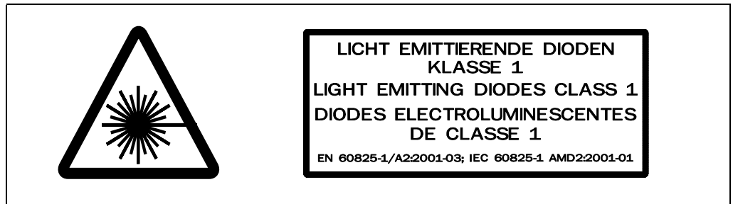
Fig. 2-1: Black-yellow signed warning labels found on the ICR
