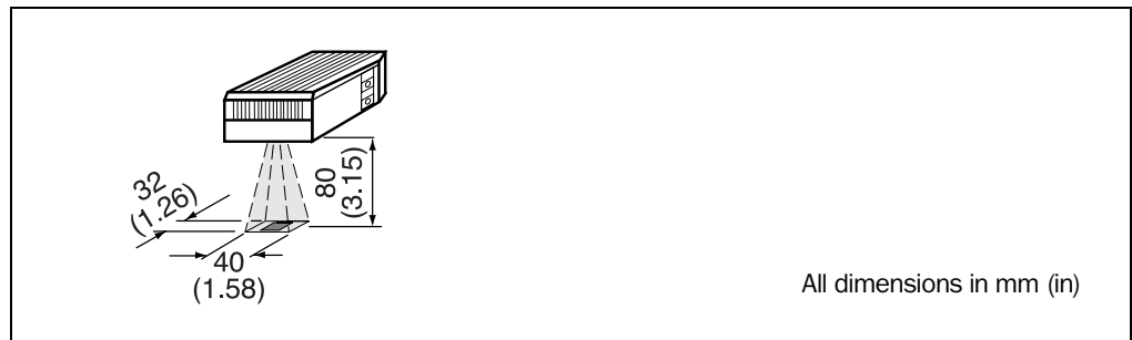
Fig. 3-2: Reading area of the ICR in the focus position (standard type)
