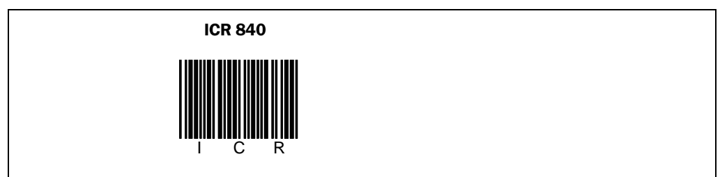
Fig. 6-2: Bar code sample (code 39; module width 0.35 mm (13.8 mil); print ratio 2:1)
