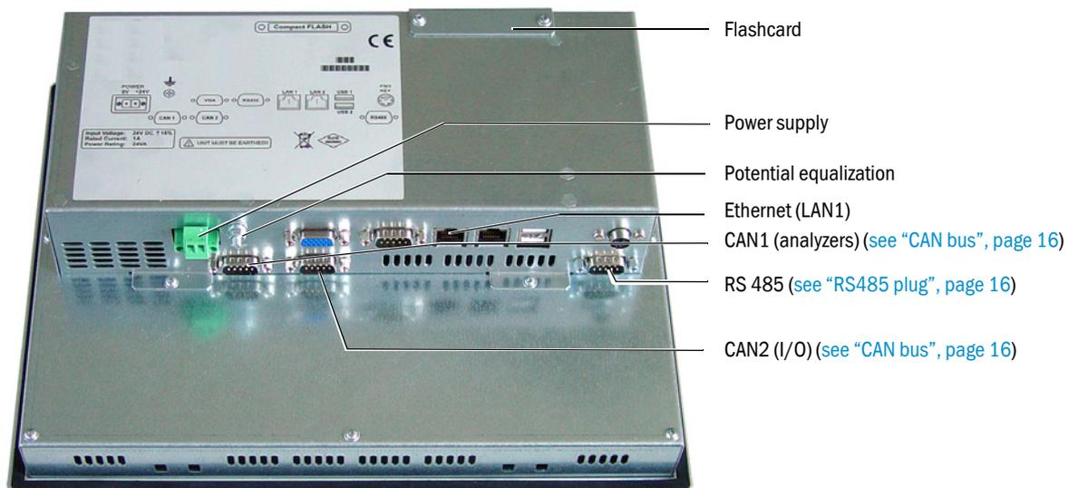
Fig. 6: Designation of connections on the back of the panel
