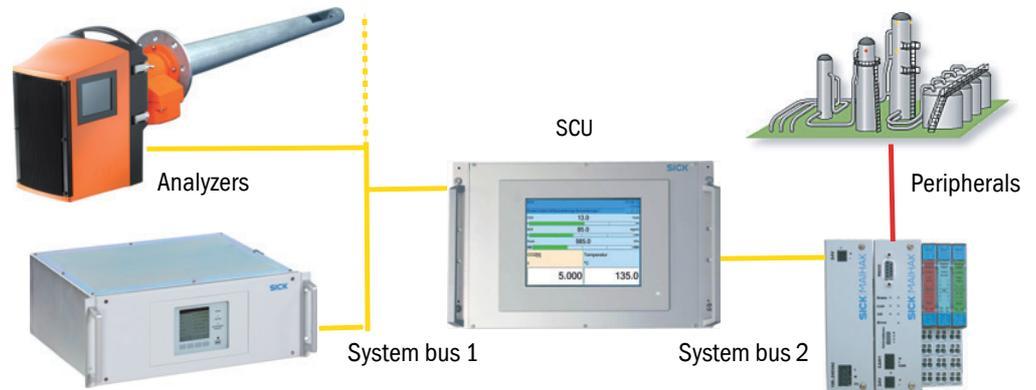
When remote control or joint control of several analyzers is used, the analyzers are connected to the SCU via a System bus. All connected analyzers are operated via the SCU. In this case, interfaces to the process peripherals are located on the SCU and additionally on the System bus (depending on the configuration).
