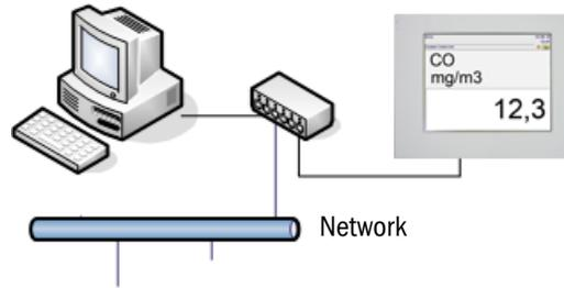
A PC and a network can be connected simultaneously to the SCU using a switch (multiple distributor) or hub.
