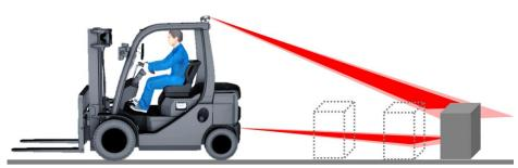
Fig. 20: Elimination of blind spot by second 2D LiDAR sensor
