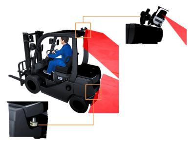
Fig. 19: Additional mounting position of a second 2D LiDAR sensor - bottom
