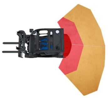
Fig. 22: Monitoring the rear area as well as the side areas
