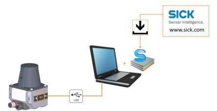
Fig. 42: Connecting 2D LiDAR sensors to configuration PC (USB)
