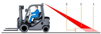
Fig. 15: Correctly setting the tilt angle of the top-mounted 2D LiDAR sensor
