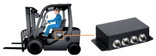
Fig. 29: Mounting the control unit on the driver's seat
