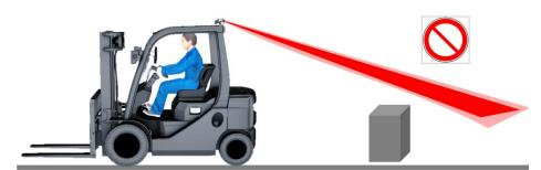
Fig. 17: Tilt angle of the 2D LiDAR sensor too flat
