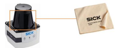
Fig. 43: Cleaning the front screen of the 2D LiDAR sensor
