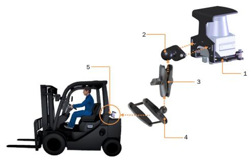
Fig. 28: Example of mounting with RAM MOUNT universal brackets
