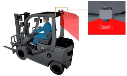
Fig. 14: Mounting position of the 2D LiDAR sensor - top
