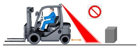
Fig. 16: Tilt angle of the 2D LiDAR sensor too steep
