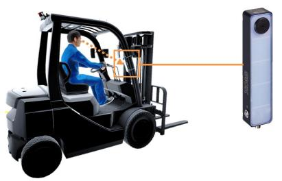
Fig. 30: Mounting the signal light bar(s) in the driver field of vision
