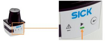
Fig. 41: Reading the operational readiness on the 2D LiDAR sensor
