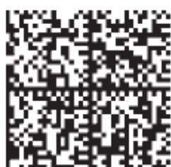
**Fixed Pattern Damage – According to ISO/IEC 15415**
