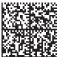
**UEC – Unused Error Correction – According to ISO/IEC 16022**
