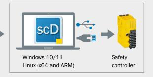
Step 2: Transfer the verified configuration to the safety controller with Safety Configuration Deployment.
