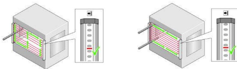
**Devices with deactivated restart interlock:** If the field indicator or integrated LED on the receiver lights up green, even if only briefly, work must stop at the machine.
