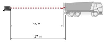
Without a filter: The LiDAR sensor detects and processes all received signal values.
