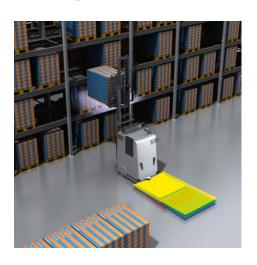
Smooth processes are essential in high-bay warehouses. Free storage spaces must be filled quickly and without complications. The MRS1000 enables exact positioning of transport forks in automated guided vehicle systems (AGVs), making collision-free movement into a free space possible. When moving backwards, the MRS1000 detects objects protruding into the space with its several scanning layers, ensuring reliable collision protection.
