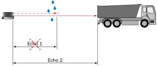
With a filter: The LiDAR sensor blanks unwanted echoes from ambient conditions in accordance with the specifications.
