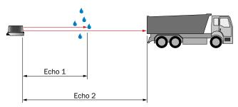
Without a filter: The LiDAR sensor receives unwanted echoes from ambient conditions such as rain.
