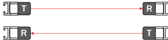
Figure 10: Light grid installed in opposite directions R = Receiver; T = Transmitter (sender)
