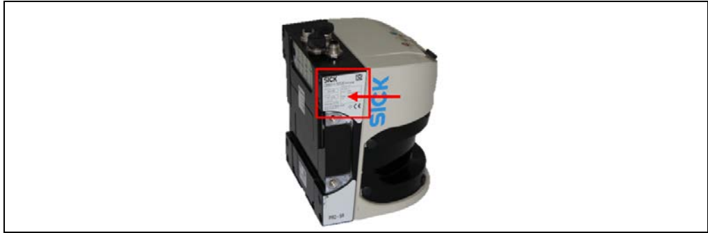
Fig. 73: Mounting the LMS Axle – noting serial numbers of the 2D LiDAR sensors
