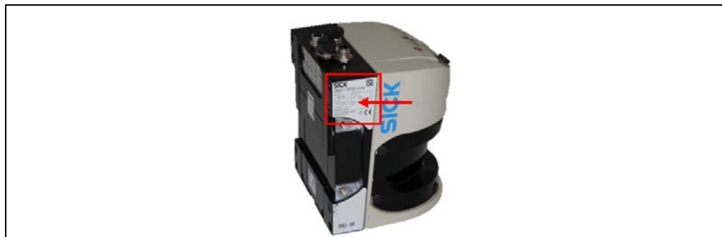
Fig. 71: Mounting TIC501 – noting serial numbers of the 2D LiDAR sensors
