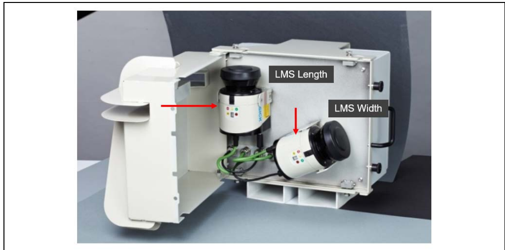
Fig. 66: Mounting the TIC102 – Noting serial numbers of the 2D LiDAR sensors
