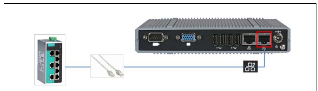
Fig. 91: Electrical installation of the TIC502 / TIC501 – Connecting the Traffic Controller to the Ethernet switch
