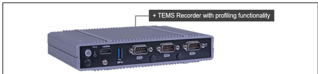
Fig. 3: Traffic Controller as the central control unit of the profiling system
