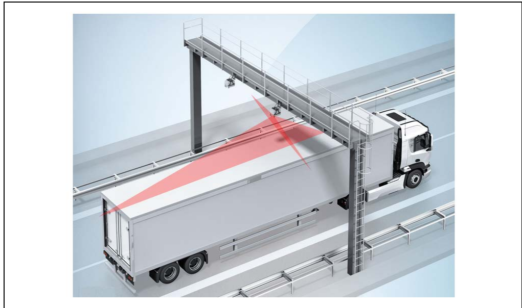
Fig. 21: Vehicle detection operating principle – detection of vehicle contour
