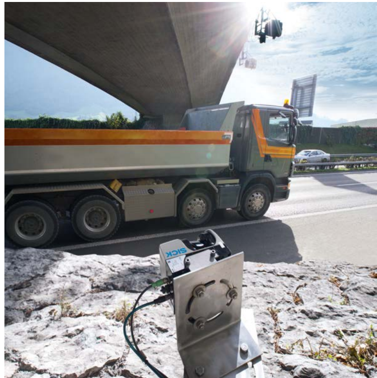
Axle counting with a 2D LiDAR sensor mounted at the roadside
