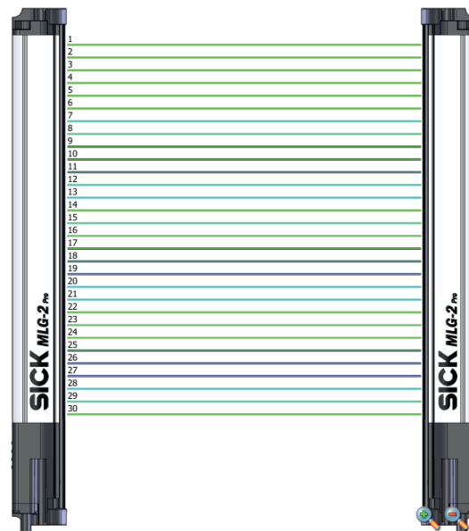
Figure 96: Beams highlighted in color in the simulation
