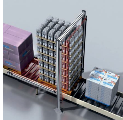
Figure 20: Detection of transparent objects
