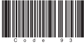
Fig. 2-7: Example of Code 93
