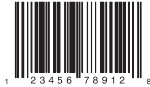
Fig. 2-4: Example of UPC
