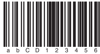
Fig. 2-8: Example of Code 128
