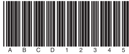
Fig. 2-3: Example of Code 39
