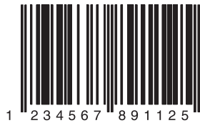
Fig. 2-5: Example of EAN 13
