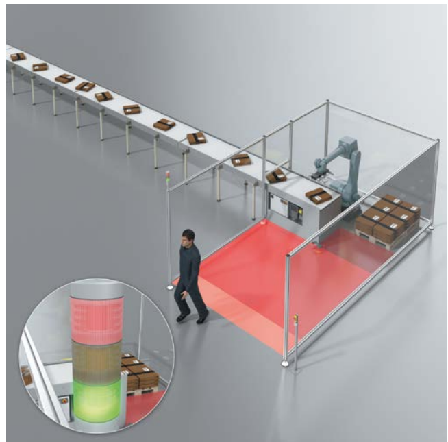
4 As soon as the person leaves protective field 1, the robot automatically restarts after successful testing the safe sequence monitoring*. Manual restart of the robot is only required if the person does not correctly follow the expected exit sequence or enters protective field 3.
