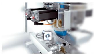
The cutting and separation of the tube bags after the sealing process causes mechanical shocks that act on the ball bearing in the servo motor of the packaging machine. The motor feedback system measures these vibrations. If they reach a threshold, an alert is triggered. This makes it possible to plan the maintenance of the servo motor and avoid unplanned machine downtimes.
