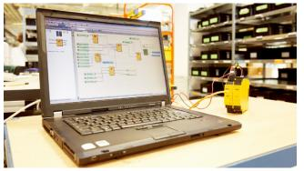
Thanks to its magnetic operation, the RE1 offers more protection against manipulation than electro-mechanical safety switches and helps considerably lower the risk of accidents. In combination with the appropriate safety function block in the controller, the RE1 can achieve performance level e.
