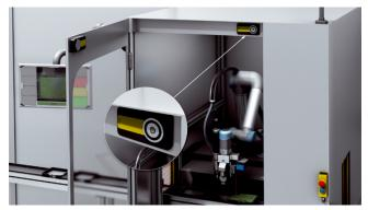
The high locking force of the electromagnet ensures that the protective door cannot be opened on accident.
