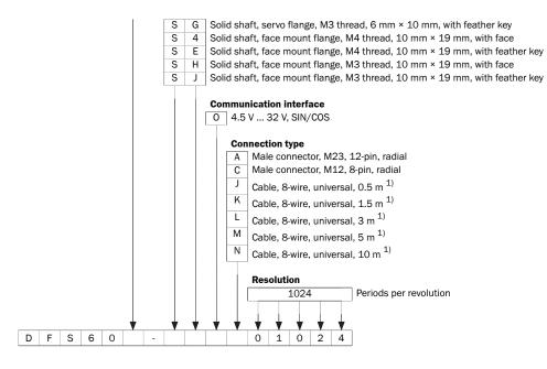
1) The universal cable outlet is positioned so that it is possible to lay it without bends in a radial and axial direction. UL approval not available.
