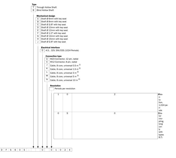
1) The universal cable outlet is positioned in such a way that kink-free laying in radial or axial direction is possible. UL-certificate not available.
