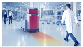
Adaptive safety concepts with Safe Motion functions ensure safe collaboration between humans and mobile robots, even in situations where space is limited.
