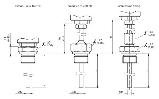
Dimensional drawing: conical threads
