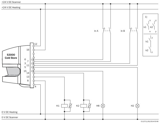
S3000 Cold Store in conjunction with relays/contactors Protective field switching by means of control inputs A and B  $\,$
