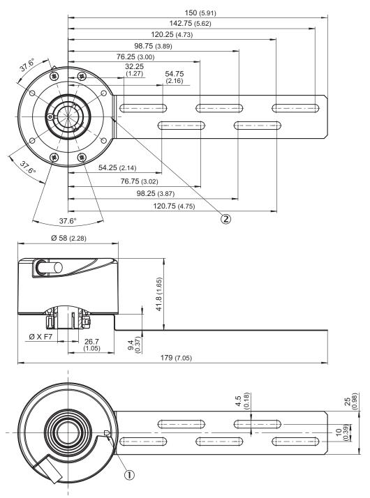
XF7 values see shaft diameter table for through hollow shaft, clamping at the front
