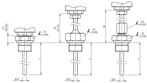
Dimensional drawing: conical threads
