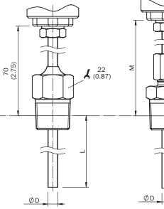
Dimensional drawing: housing, without process connection
