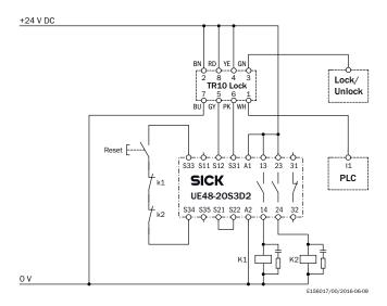
Series connection of three TR10 Lock safety locking devices to a Flexi Classic safety controller
