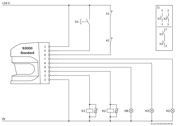
S3000 Standard in conjunction with relays/contactors
