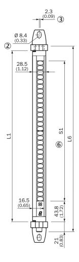
Sender with swivel mount, small housing (receiver mirror image)
