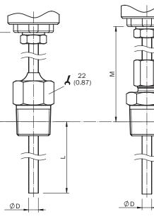
Dimensional drawing: housing, without process connection
