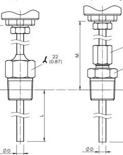
Dimensional drawing: housing, without process connection
