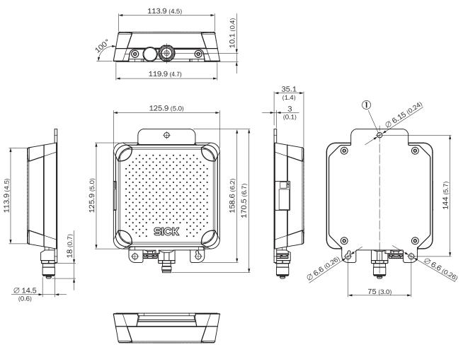
① Mounting hole for M6 screws (3 x)
