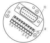
① Internal plug connector to encoder
