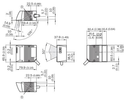
① Blind hole thread M5, 5 mm deep (2 x), for mounting
