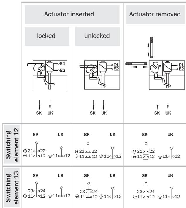
⬇ Positive action N/C locking monitoring contact
