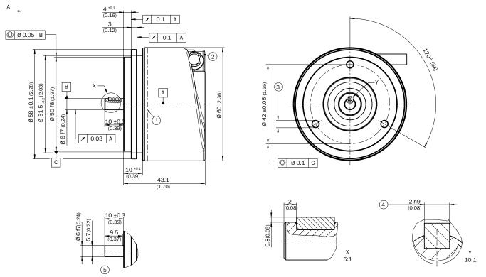
① Operating temperature measuring point (freely selectable, around the housing surface area in each case, approx. 3 mm away from flange)
