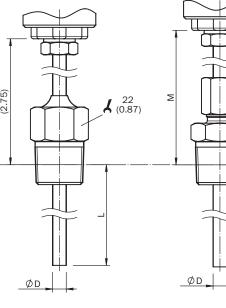
Dimensional drawing: housing, without process connection
