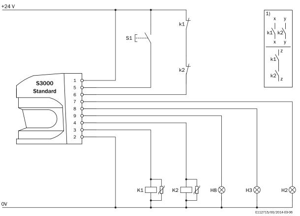
S3000 Standard in conjunction with relays/contactors
