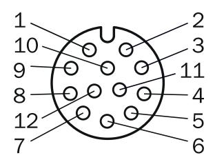
M12, 12-pin female connector, A-coded (I/O)
