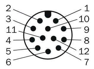
M12, 12-pin male connector, A-coded
