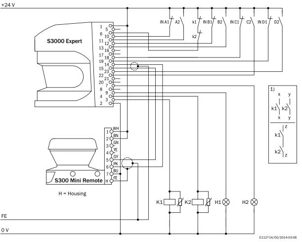
${\tt S3000 \ Expert \ with \ S300 \ Mini \ Remote \ in \ an \ EFI \ system \ with \ relays/contactors}}$
