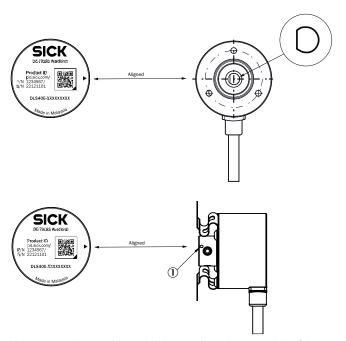
You can see the position with the mark on the rear side of the encoder ① Zero pulse mark on housing
