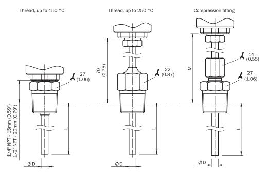
Dimensional drawing: housing, without process connection
