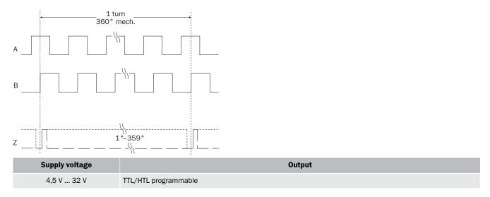
Electrical zero pulse width can be configured to 90°, 180°, or 270°. Width of the zero pulse in relation to a pulse period.
