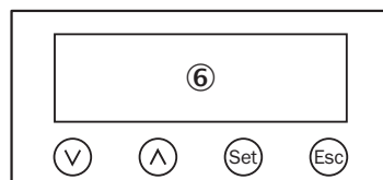
⑥ Liquid crystal display with function keys
