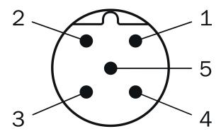
Male connector M12, 5-pin, A-coded
