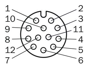
M12, 12-pin female connector, A-coded (I/O)
