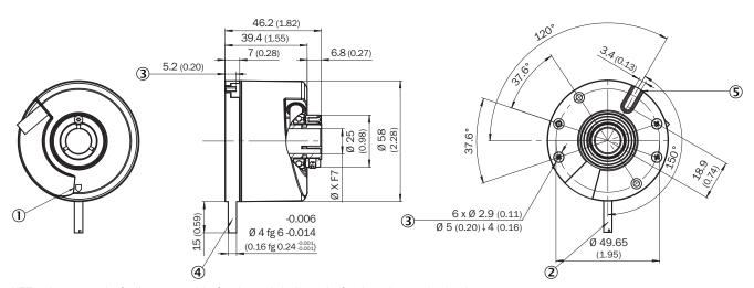
XF7 values see shaft diameter table for through hollow shaft, clamping at the back
